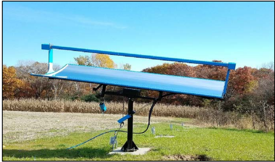
Meet LEMA, one of five solar-powered water pasteurization units to be installed on the Ruth Gaylord Hospital campus.
